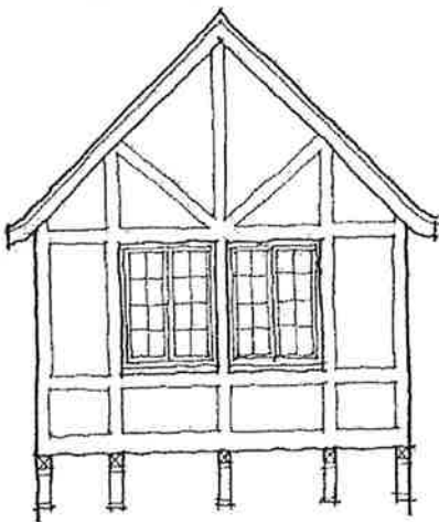
Typical Cantilevered Gable
