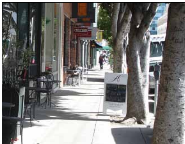
Sidewalk sign located to maintain accessible route.
