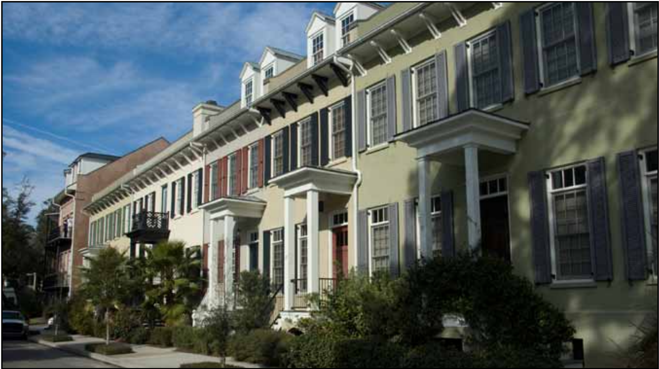
Individual stoops and dormers help to break down the overall massing of this row of townhouses.
